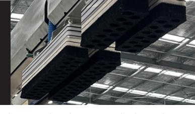
The latest Version of the Vekta PackFeeder, can now pick up to two boards at a time and is designed to pick far faster than the typical requirements of a saw- allowing it to pick for multiple saws. When combined with a Stak-n-Gap, the system can automatically flip boards for bow and stack lumber on top of one another. When combined with a Razer saw, even greater benefits are realised with seamless, product specific software to really take full advantage of this amazing product.
